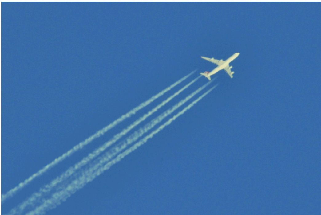
This picture shows the contrail (condensation trail) left behind by a jet. Water vapor in its exhaust gases condense on dust particles in the air.
